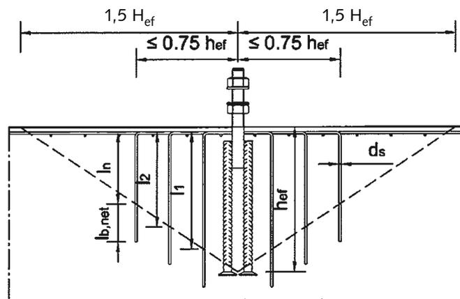
Fig. 8: Example for the arrangement of the suspension reinforcement, for which the dimensioning of a surface reinforcement is required
