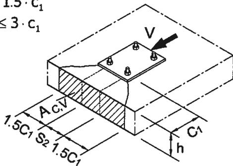
a) Group of Anchor Bolts at the edge of a thin structural element
