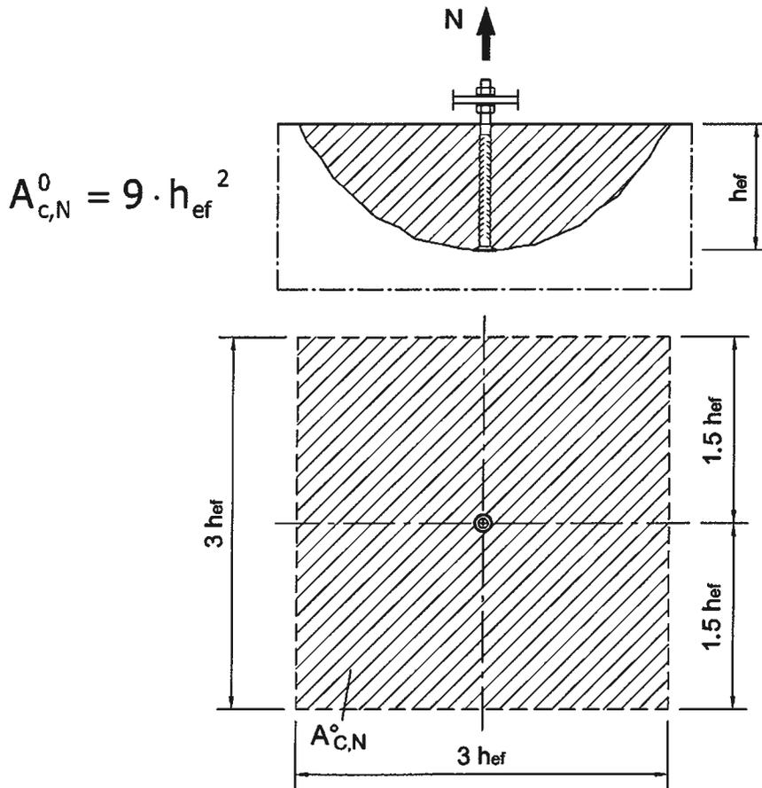
**Figure 7: Example for the available area of the idealised concrete blow-out body under tensile stress from the Anchor Bolts**
