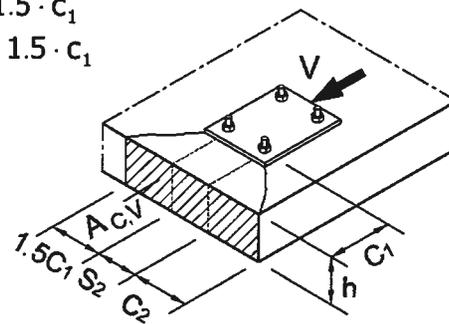
a) Group of Anchor Bolts at the corner of a thin structural element
