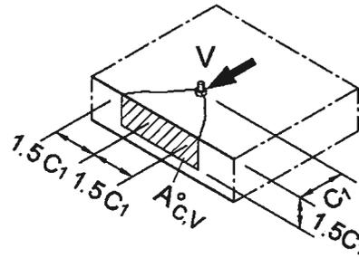
**Fig. 12: Examples for present areas of the idealised concrete blow-out bodies for Anchor Bolt groups under transverse stress**
