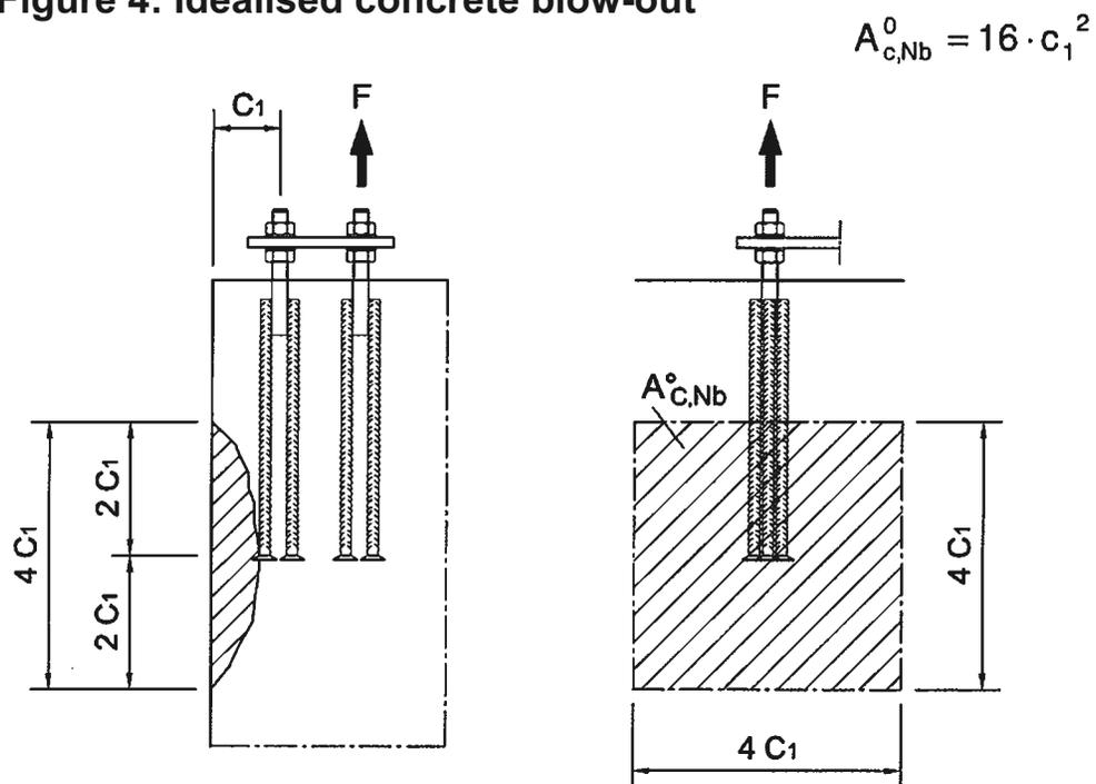
**Figure 5: Example for a local concrete blow-out at the edge**
