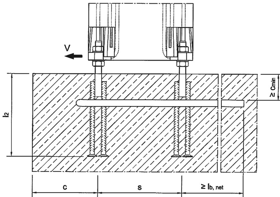
$c_{min}$ ,  $l_{b,net}$  and  $d_{br}$  acc. to DIN 1045-1
